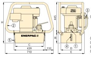
User adjustable relief valve on all manual valves. 3/8" NPTF on A and B ports; 1/4" NPTF on auxiliary ports.
